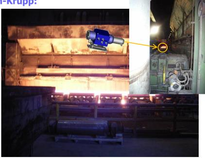
Further more LMC-FUR-50 are used at inlet side for length positioning as well as charging positioning of the slabs.
